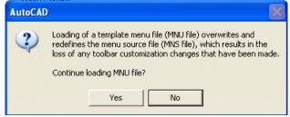
Click on load button. Click yes to continue. For latest version, Click on close. 2d menu will be loaded, and start using pull down menu. The pull-down menu, has all the 2D piping model drawing options. The other menu items are not modified.
