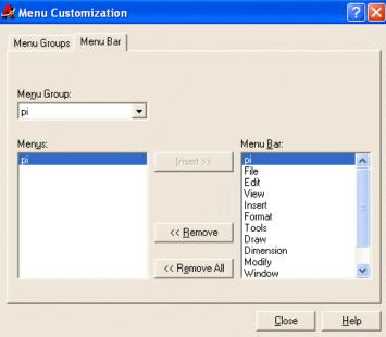
Click on insert and then click on close button. 2d menu will be loaded, and start using pull down menu. The pull-down menu, 2d has all the 2D piping drawing options. The other menu items are not modified.
