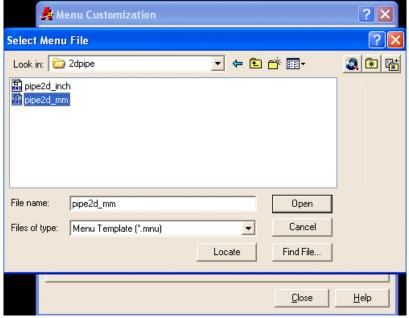
Change folder to the folder where all program files are located and click on arrow of Files of Type box. Select Menu Template (\*.mnu) and select pipe2d\_mm or pipe2d\_inch as menu to be loaded. Click on open button.
